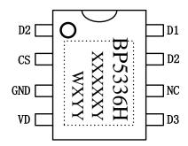
Fig. 2 Pin Configuration
